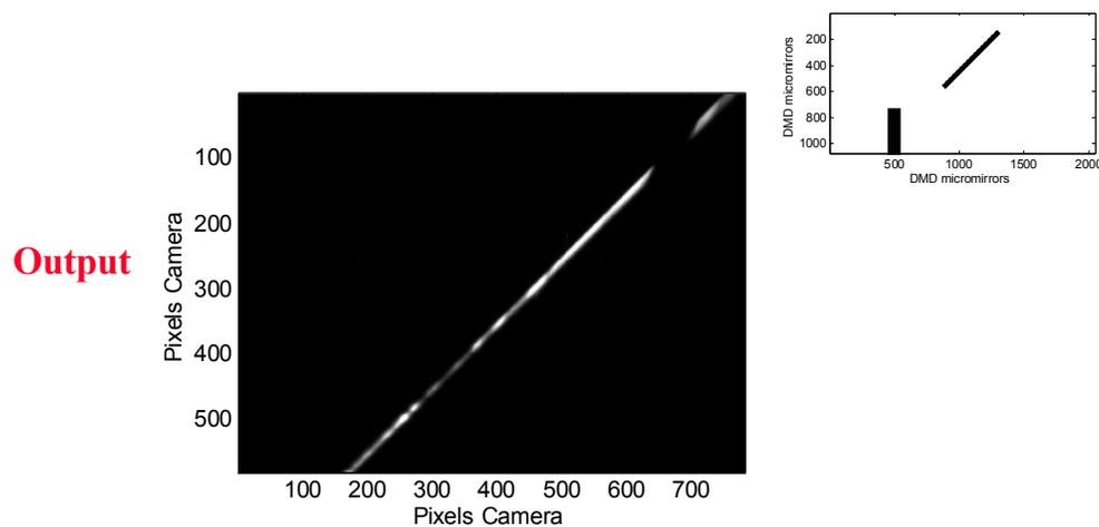
**Fig. 8.** End-to-end measurement: image recorded at the output of the programmable spectrograph; the bright object and the diffraction 0<sup>th</sup> order light are removed. DMD surface behavior is shown (black pixels are OFF)
