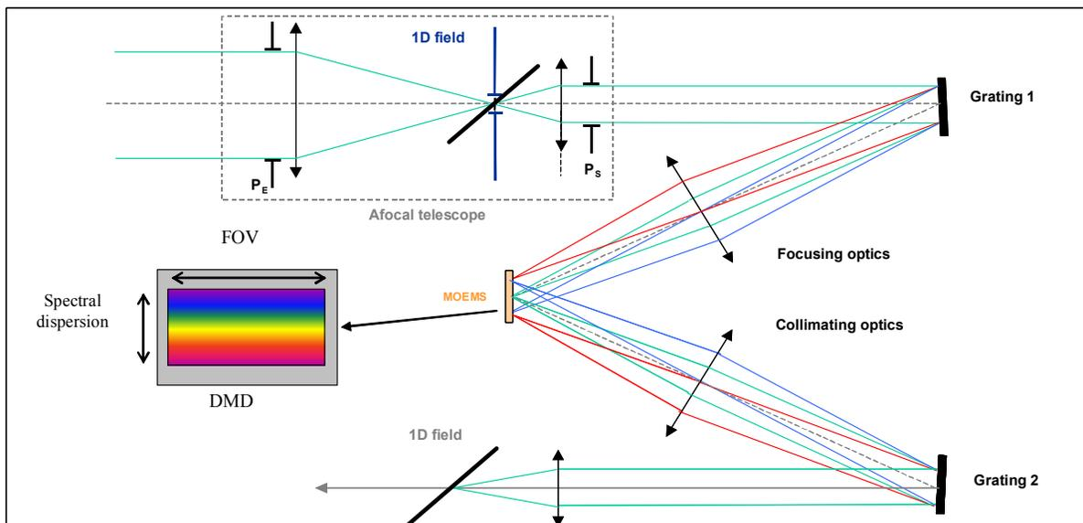
**Fig. 1.** Principle of the programmable wide-field spectrograph using a MOEMS device (DMD from TI) for wavelength tailoring on each field pixel.
