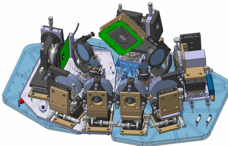
**Fig. 3.** Opto-mechanical design of the programmable wide field spectrograph, 3D general design view
