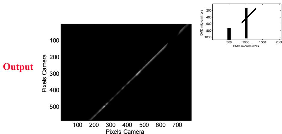
**Fig. 9.** End-to-end measurement: image recorded at the output of the programmable spectrograph; the bright object, “blue” color along the whole 1D image and the diffraction 0<sup>th</sup> order light are removed. DMD surface behavior is shown (black pixels are OFF)
