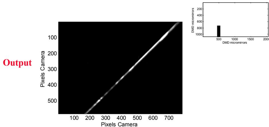
**Fig. 7.** End-to-end measurement: image recorded at the output of the programmable spectrograph with all DMD pixels ON except those removing 0<sup>th</sup> order light. DMD surface behavior is also shown (black pixels are OFF)
