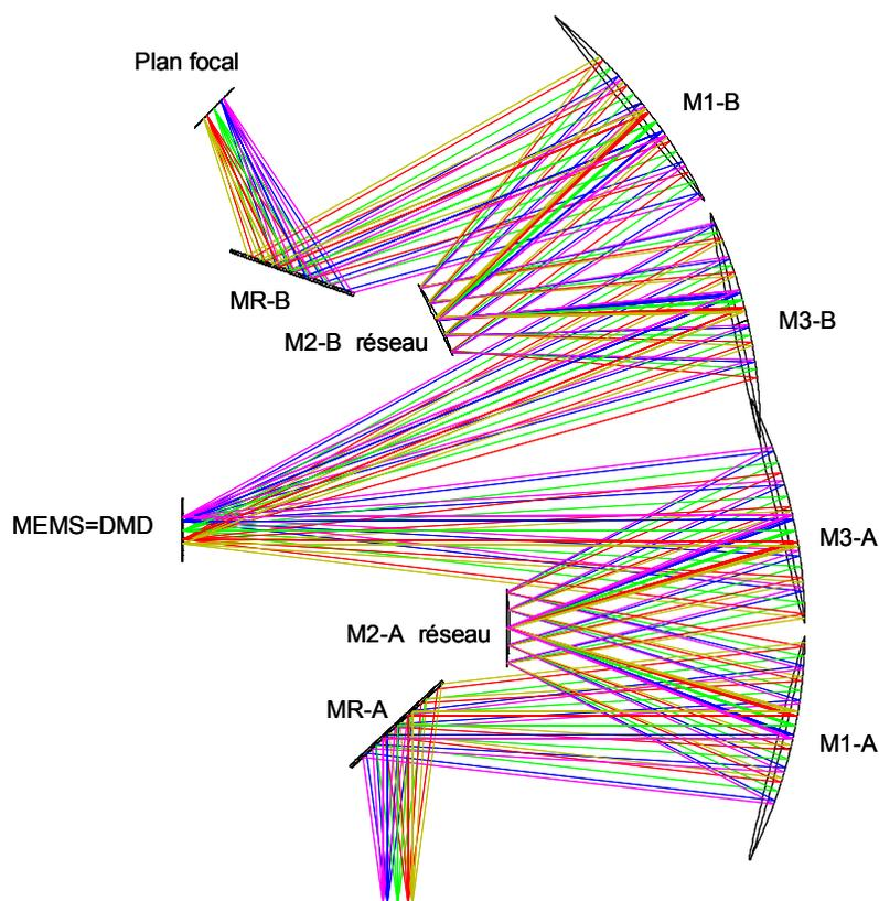
**Fig. 2.** Optical design of the programmable wide field spectrograph demonstrator. Light from the telescope is coming from below (1D entrance slit), passing through two Offner-type spectrographs in serial separated by the DMD, up to the detector at the top of the drawing.
