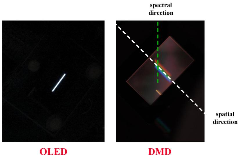
**Fig. 5.** Images of the input (OLED) plane and intermediate focal plane (DMD surface).
