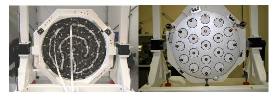
Fig 1 OBB Backplane final assembly. Left: back view. Right: front view on the optical bench test stand.
