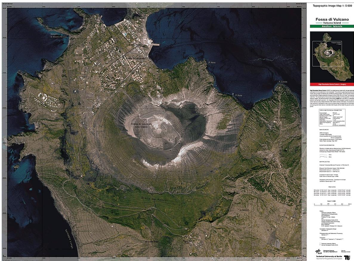
Figure 4. Topographic Image Map Fossa di Vulcano 1: 5,000. Color orthoimage mosaics, contour lines, and spot heights have all been derived from HRSC-A stereo imagery.
