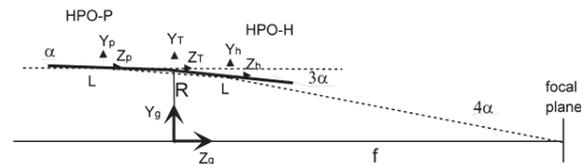
Fig. 4. One mirror layout of the TANDEM with coordinate systems of the telescope, TANDEM, HPO-P and HPO-H
