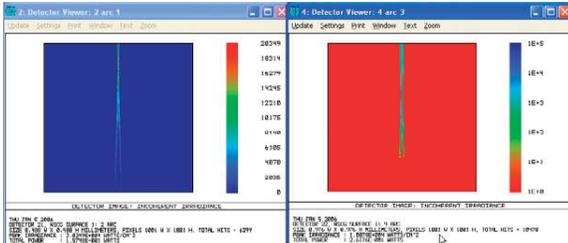
Fig. 10. Spot image in focal plane for TZ = -5 mm
