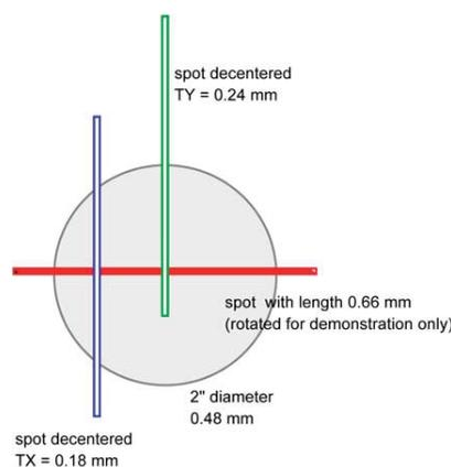
Fig. 6. Focal plane simulation of the current Tandem
