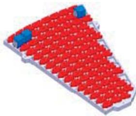
Fig. 3. FFF Model Petal with 3 optical Tandems
