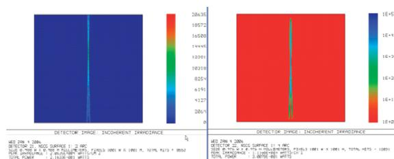
Fig. 5. Spot image in focal plane with 2" x 2" (left, linear scale) and 4" x 4" (right, log scale) detectors
