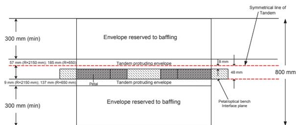
Fig. 2. Axial envelope cross section
