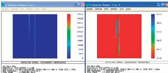
Fig. 11. Spot images in focal plane for two different tolerances, RX = 205'' and RY = 1850''
