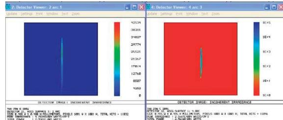
Fig. 12. Spot image in focal plane for RY = 1850'' compensated by TX = 70 μm and TY = 240 μm
