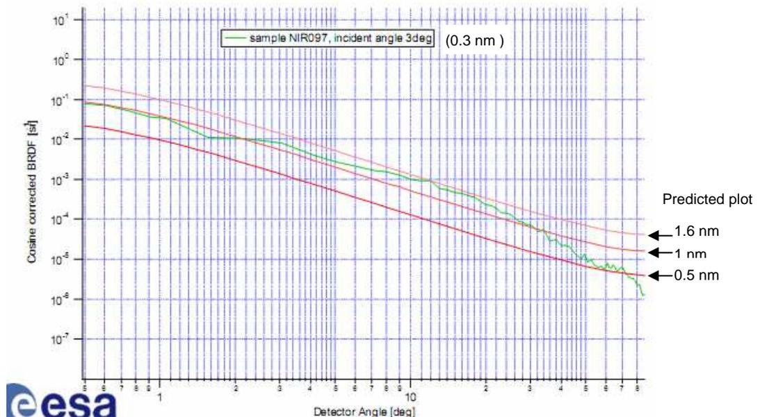
Figure 7: Comparison between actual BRDF measurement and prediction with Dittman model
