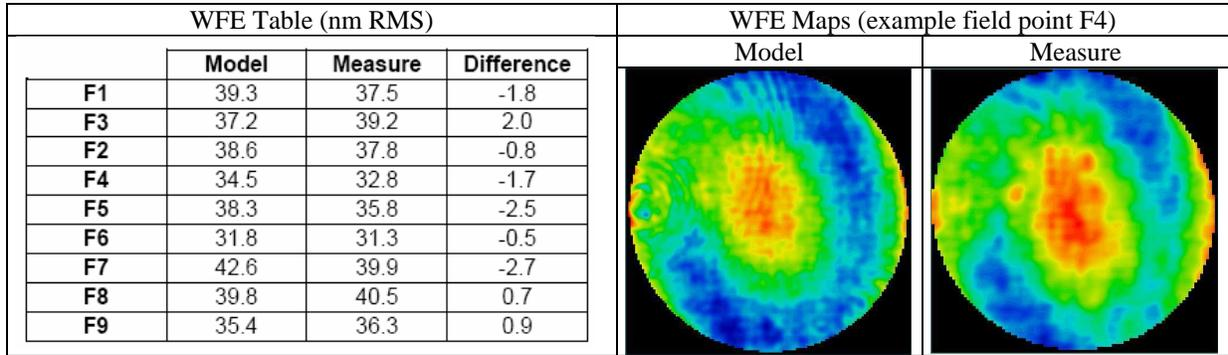
Figure 4 : As built model : fit of WFE measurement
