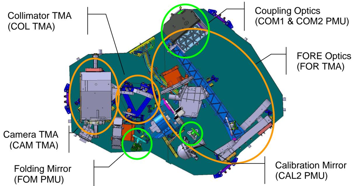
Figure 1 : Top view of the NIRSpec instrument with Sagem contribution
