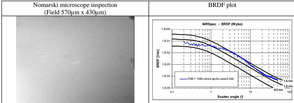
Figure 6: Process performance for Flight Model mirror ( $\mu$ -roughness 0.4 nm)
