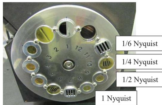
Fig. 8. Four-bar targets mounted on the collimator system
