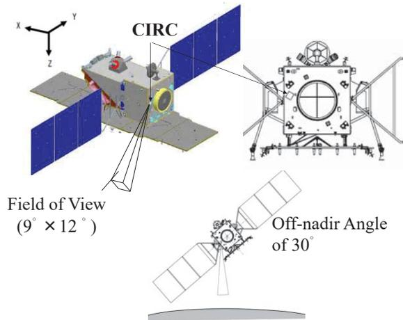
Fig. 2. Schematic view of ALOS-2
