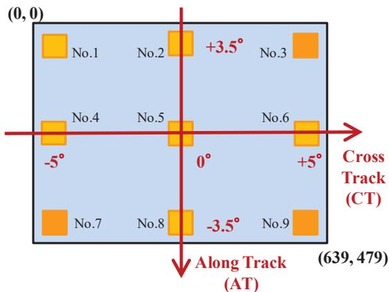
Fig. 10. Measurement points of MTF on image acquired by CIRC
