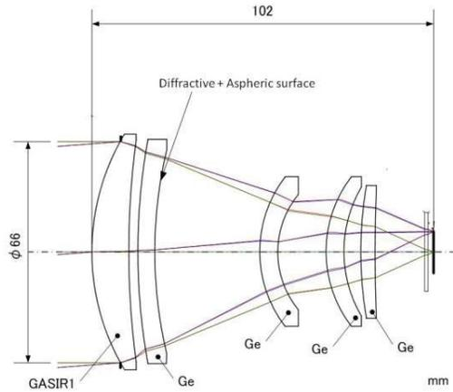
Fig. 5. Optical design of the CIRC
