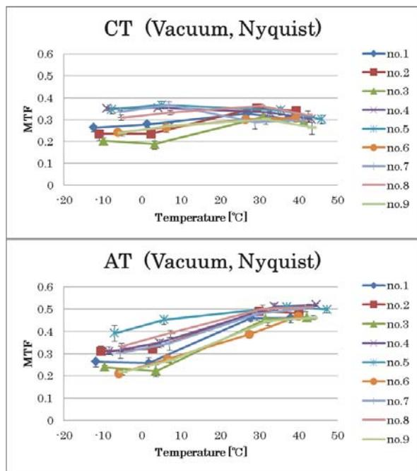
Fig. 12. Measurement results of MTF. MTF in the CT direction (top). MTF in the AT direction (bottom)
