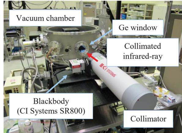
Fig. 7. Experimental setup of MTF measurement
