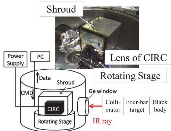
Fig. 6. Schematic view of MTF measurement
