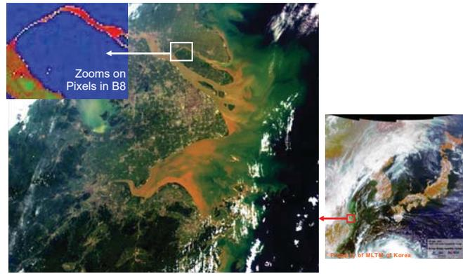
Fig. 15: Shanghai Yangtze River, China, from raw data. The close-up on one slot shows streets detail (theoretical GOCI is resolution 500m at this latitude). An additional zoom shows the B8 pixels demonstrated the detection of sharp contrasts.
