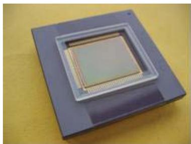
Fig. 6: GOCI CMOS Detector
