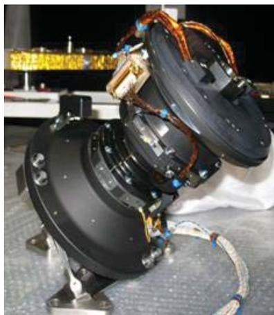
Fig. 7: GOCI Pointing Mechanism (w/o mirror)
