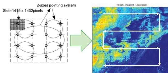
Fig. 5: Principle of GOCI image acquisition
