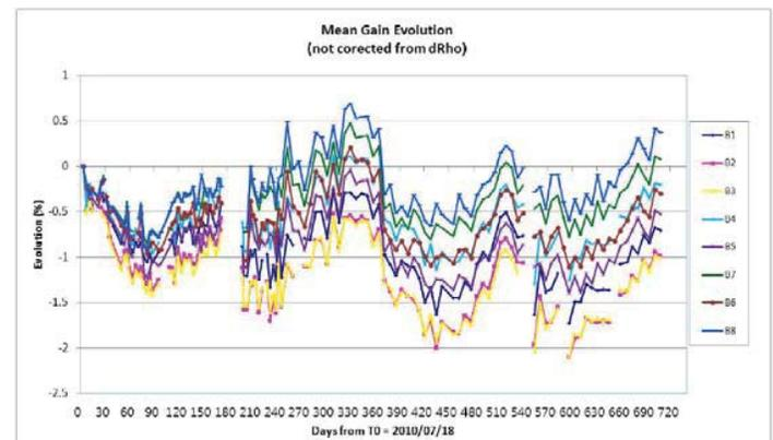
Fig. 18: Evolution of gain computed through GOCI in-orbit calibrations during the first 2 years.
