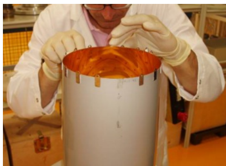
Fig. 6. Shell under preparation for integration
