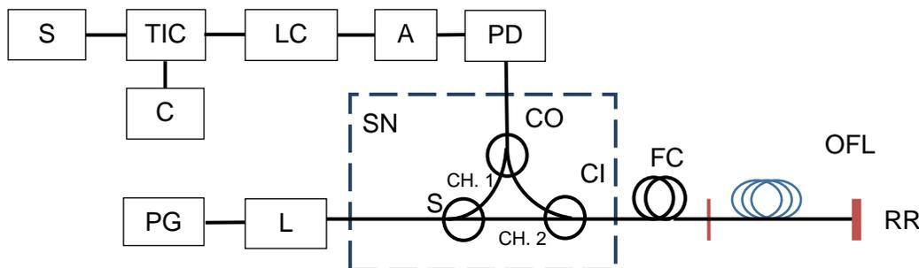
Figure 1. Scheme of optical time domain reflectometer. S – frequency standard, TIC – time interval counter, C – computer, PG – pulse generator, L – laser, LC – logical converter, A – amplifier, PD – photodetector, SN – splitter node, S – splitter, CO – coupler, CI – circulator, FB – fiber coil, FOL – fiber optical link, RR – retroreflector.
