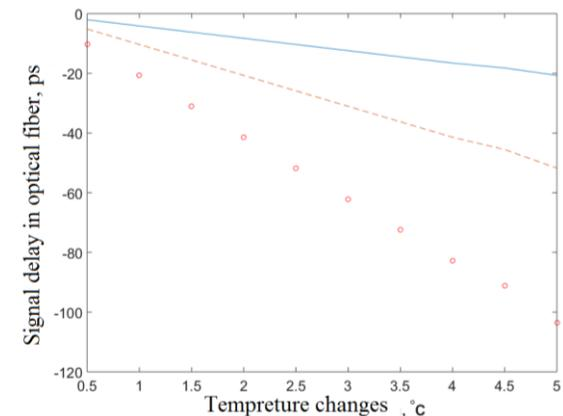
Figure 2. Changes in the propagation delay of a signal in a FOCL depending on the ambient temperature.
