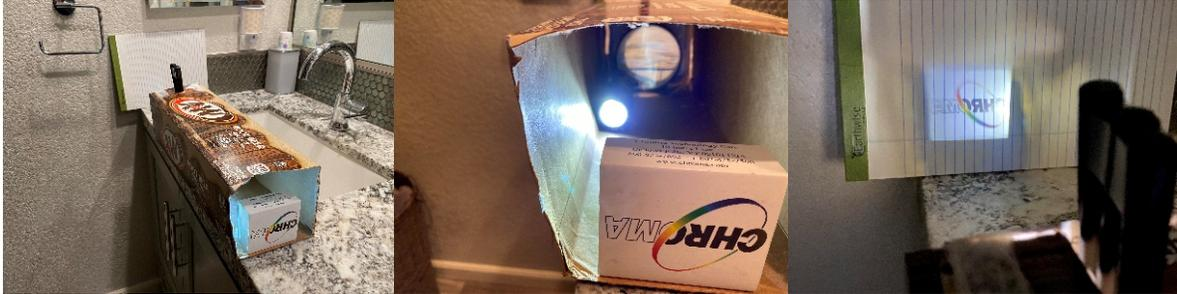
Figure 20. Light Box with Three \$1 Magnifying Glasses and a 500 Lumen Flashlight.
