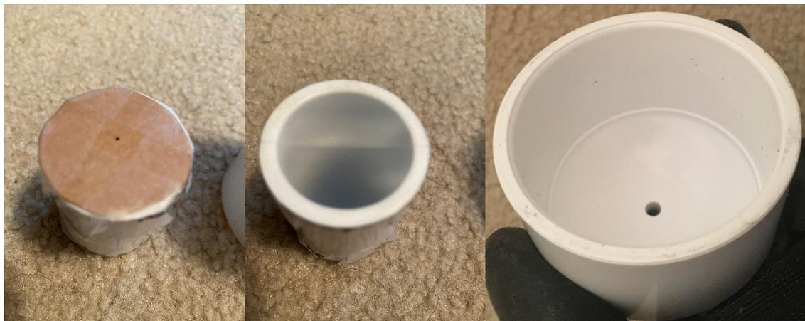
Figure 17. PVC Coupling and PVC Cap Pinhole Cameras (no Scotch Tape on Cap for Clarity)
