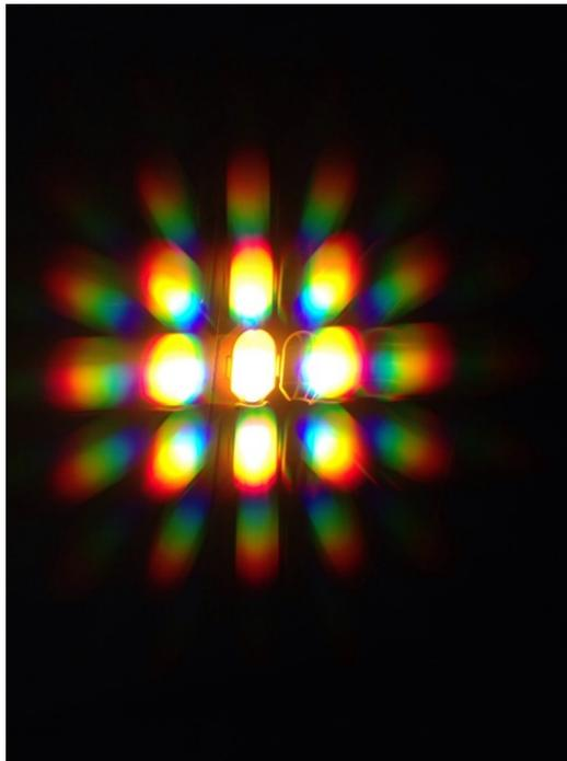
Figure 6. Picture of a Light Bulb Through SPIE Diffraction Glasses (Submitted by a Photonics Club Student).
