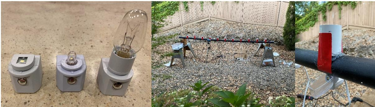
Figure 22. LED Night Light (left) Detects a Golf Ball Rolling Slowly in a Pipe.
