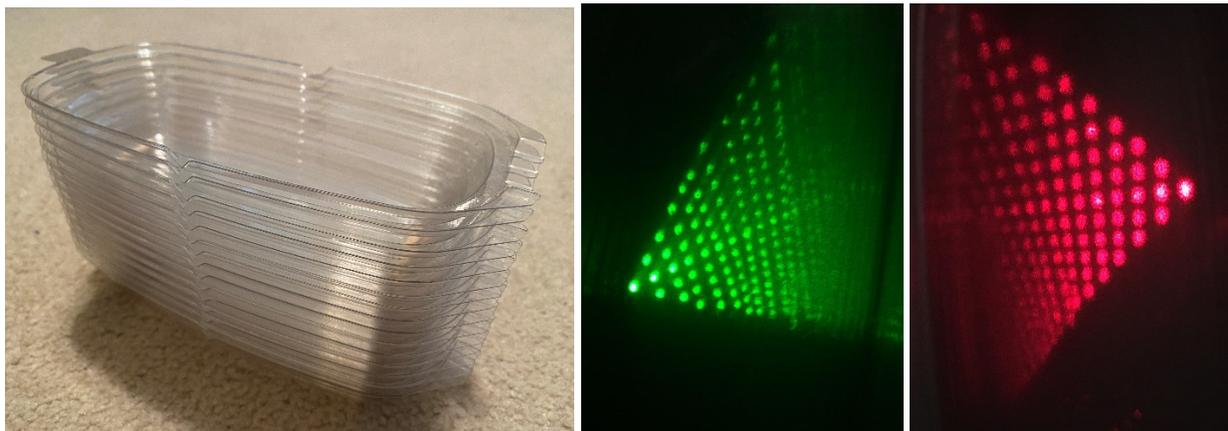
Figure 23. Reflections of Reflections Using 15 Plastic Banana Split Boats and Two Laser Pointers.
