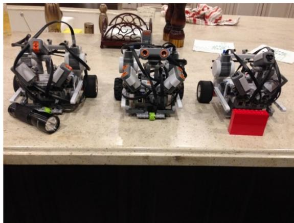
Figure 10. Lego Robots Controlled by Light (Left), Distance. (Middle), and Color (Right).
