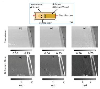
Figure 2. Anti-solvent crystallization of glycine in ethanol. 2(a) Shows a schematic of the experimental setup. 2(b)-(d) transmission images at three different points of a time lapse series. We can see the crystal formation at the edge of tubing and later at the mixing zone. 2(e)-(f) Differential phase contrast images at same intervals forming a thin-layer in the mixing zone.
