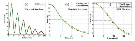
Figure 1. (a) Visibility measurement for pink beam. 1.1(b-c) coherence measurement for filtered X-ray pink beam and MLM Mo/B<sub>4</sub>C stripe.
