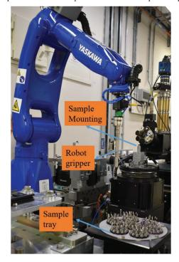
Figure 4. Picture of the sample changer robot installed in the I13-2 Diamond-Manchester Imaging Branchline.
