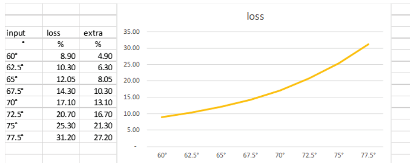
Figure 10 calculated extra polarization loss
