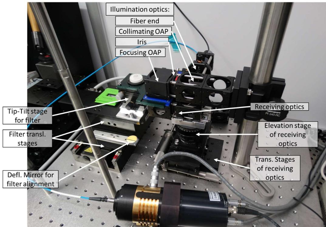
Figure 6 Front end fiber optic coupling optics and filter positioning stage (left) and Filter holder (blue) in between the optics
