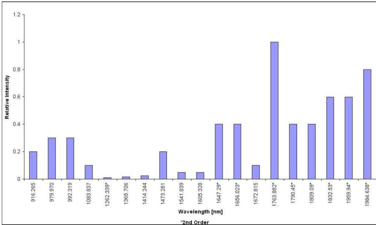
Figure 11 Xe lines as given by Ocean Insight. The lines marked with \* are not real lines, but second orders of the grating when omitting an order sorting filter
