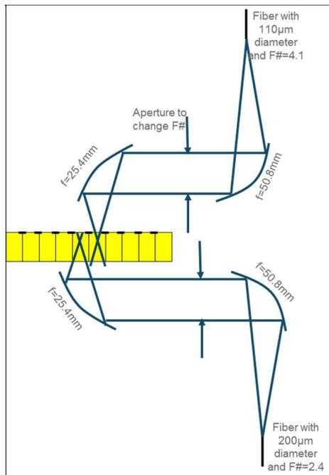
Figure 19 setup for measurement of crosstalk of the adjacent channel
