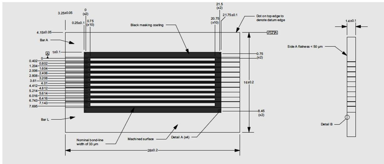
Figure 12 Geometry of filter under test – section of production drawing.
