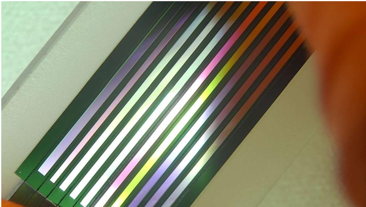
Figure 13 multispectral filter in visual inspection: glue gaps are visible as thin dark stripes, covered by the aperture mask of the filter.
