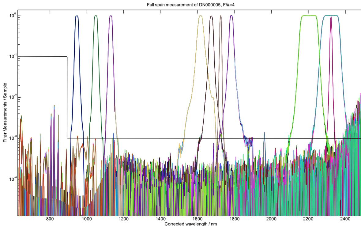
Figure 18 complete scan of all channels showing the requirement for out of band blocking as black line
