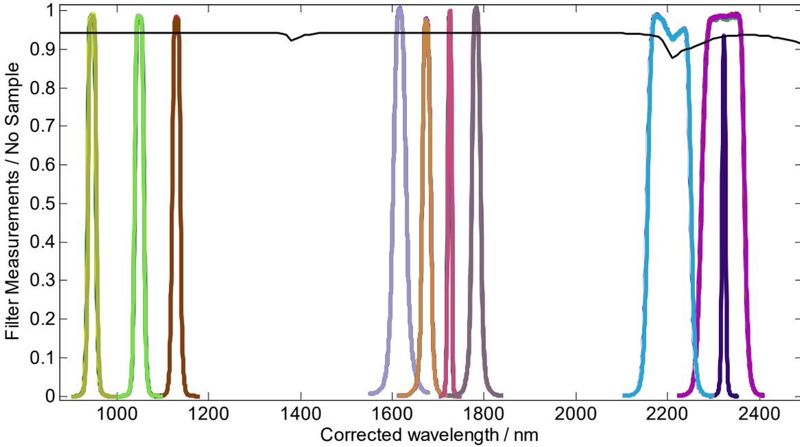
Figure 15: complete scan of all filters and substrate, measured with F# of 4.
