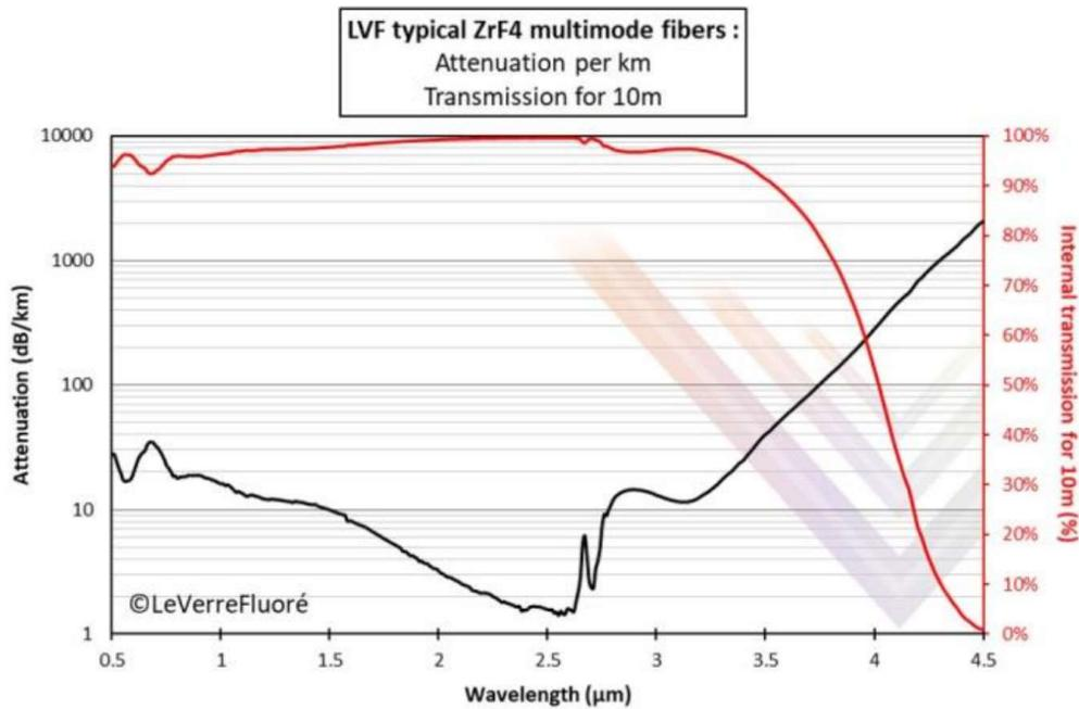
Figure 4 Transmission for a ZrF<sub>4</sub> Fiber
