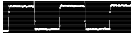
Fig. 12: Typical output signal of the ELT system. The amplitude is a measure for the change in capacitance of during switching. The slopes can be used to determine the switching speed (see Fig. 16).
