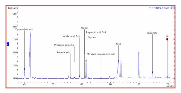
Fig. 8. GC-MS analysis of the products formed after hydrolysis at neutral pH of Titan's tholins: <u>GC conditions</u>: (column Rxt-1 (Restek) L: 30 m; Int. diam.: 0.25 mm, Temperature program:  $60^{\circ}$ C (20 min) – ramp 2°C/min until 260°C (maintained 10 min); Gas vector: He (flow: 1 mL/min) – <u>sample conditions</u>: (tholins synthesis: 60 mA; 1 mBar, 400 K) - 48 H hydrolysis in water (Millipore) at 70°C, derivatization: 30 µL MTBSTFA; 10 µL DMF.
