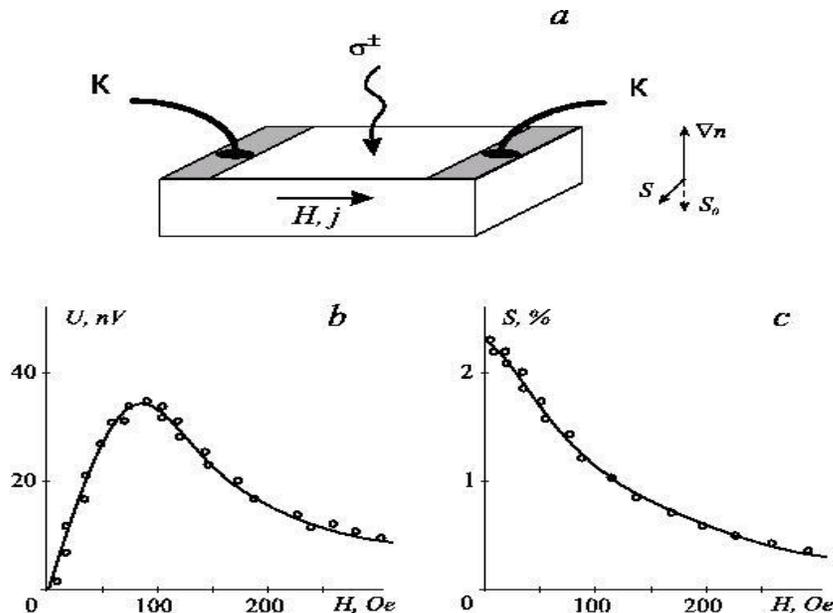
Fig. 1. First experimental observation of the Inverse Spin Hall Effect [4]. *a* - the experimental setup, *b* - voltage measured between the contacts *K* as a function of magnetic field, *c* - measured degree of circular polarization of luminescence, equal to the normal component of the average electron spin, as a function of magnetic field. The solid line in *b* is calculated using the results in *c*
