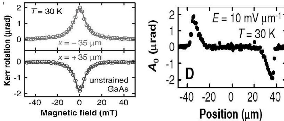
Fig. 2. First observation of the Spin Hall Effect [6]. Left panel - measurements of the Kerr rotation as a function of magnetic field at the opposing sample edges. Right panel: spatial dependence of the Kerr rotation across the channel.
