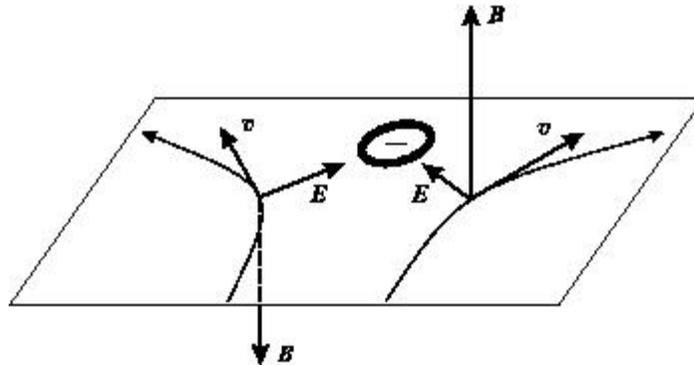
Fig. 3. Schematics of electron scattering by a negative charge. The electron spin sees a magnetic field  $\mathbf{B} \sim \mathbf{v} \times \mathbf{E}$  perpendicular to the plane of the electron trajectory. Note that this magnetic field has opposite directions for electrons scattered to the left and to the right
