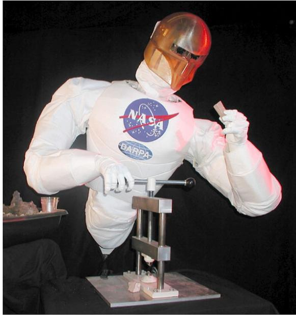
**Figure 4:** The Robonaut is remotely controlled to perform physical tasks by mirroring the actions of a human for potential future NASA missions. Courtesy of NASA Johnson Space Center.
