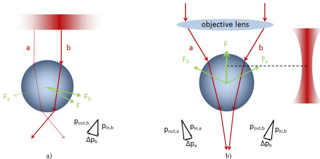
Figure 1. Optical Forces arising due to refraction at the particle surface and momentum transfer. a) Particle laterally accelerated to the point of highest beam intensity. b) Particle forced to the stable position near the beam waist.
