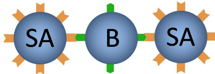
Figure 4. Simplified model for microparticle assembling using biomolecules. Complementary structures next to hydrogen bonds lead to the strong binding forces between Streptavidin and Biotin.
