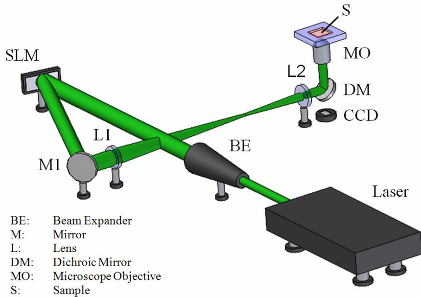
Figure 3. Experimental setup including a Yb:YAG laser (ELS – Versadisk,  $\lambda = 1030$  nm), a spatial light modulator (Holoeye Pluto NIR) and a high numerical aperture microscope objective (Zeiss Plan-Apochromat, NA = 1.4).
