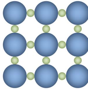
Figure 5. Model for manufacturing microstructures. Small Biotin coated particles are used as binding parts to connect the larger Streptavidin coated particles.
