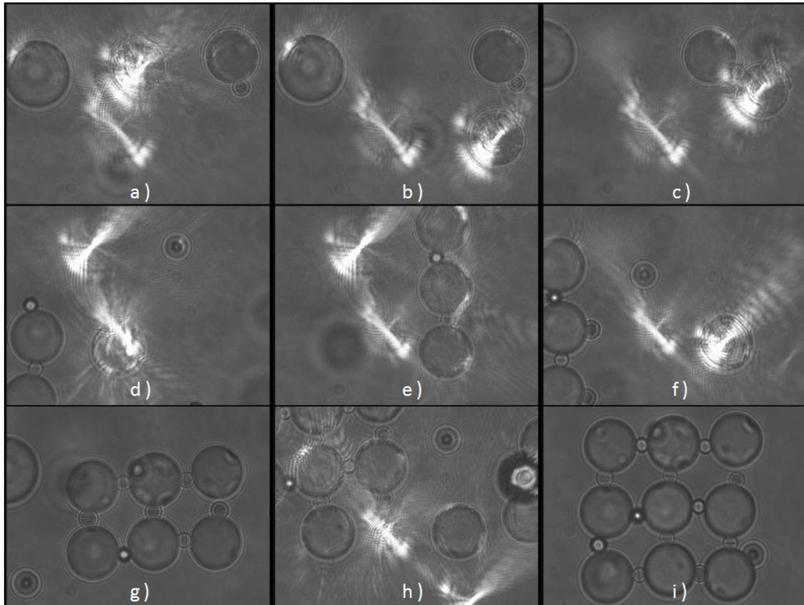
Figure 6. Micro manufacturing of a 3x3 array using Streptavidin coated polystyrene particles ( $\varnothing_{SA} = 12 \mu\text{m}$ ) and Biotin coated particles ( $\varnothing_B = 3.5 \mu\text{m}$ ) as binding parts. The laser beam position is visible due to reflection of the light at the glass water interface.
