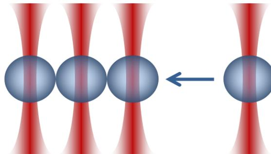
Figure 2. Micromanipulation with holographic optical tweezers. Particles can be arranged to a temporary structure. Once the laser is switched off, the particles will lose the imposed alignment.
