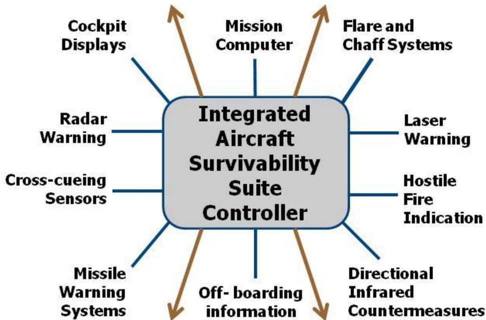
Figure 28. Integrated Aircraft Survivability Equipment Architecture
