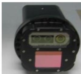
Figure 31. Northrop Grumman Advanced Threat Warner (ATW)
