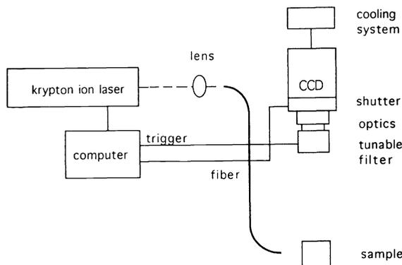
Fig.1 Set-up for spectrally-resolved autofluorescence imaging
