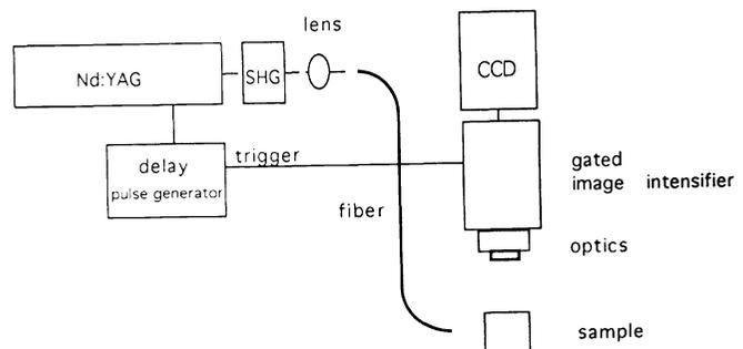
Fig. 2 Set-up for time-gated autofluorescence imaging
