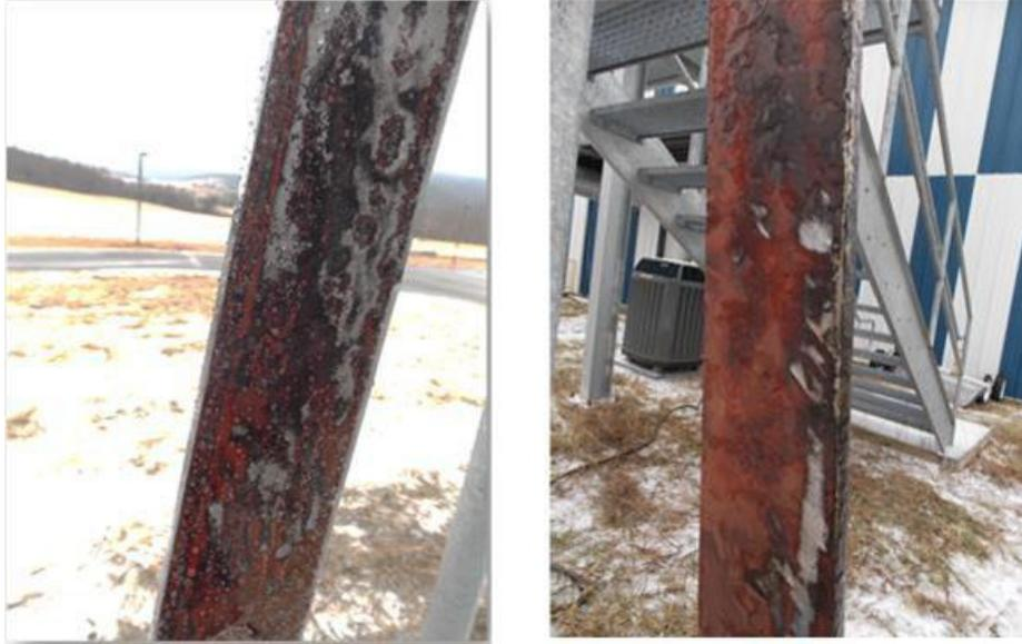
Figure 5. HybridSil icephobic-coated steel substrate (left) and uncoated substrate (right) demonstrating mitigation of ice build-up on surfaces.
