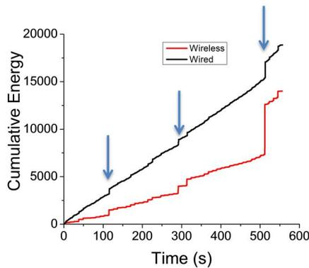
Figure 5. Cumulative AE energy as measured by the standard AE system (black) and the 1284 node (red) during the three point bending test. Notice the jumps (arrows) indicative of damage growth at different points during the test.
