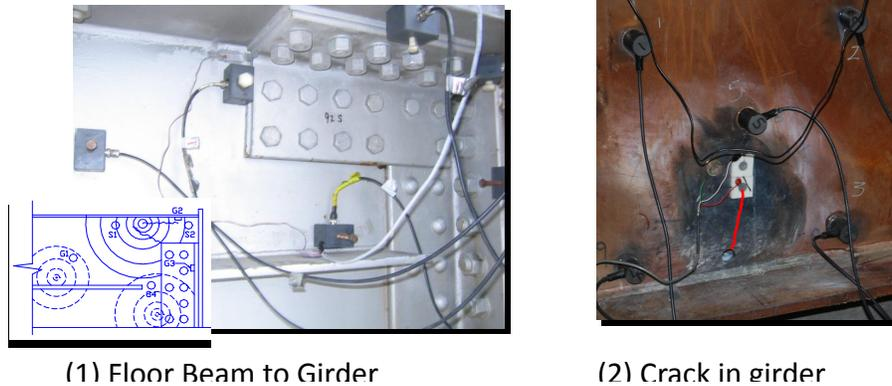
Figure 2: Examples of possible applications of critical area monitoring using the 4-channel wireless node.
