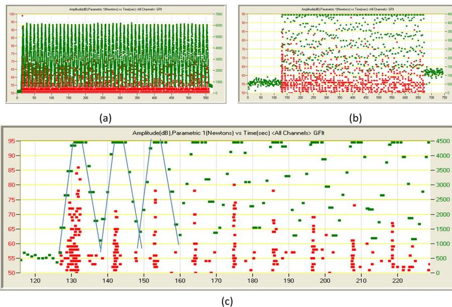
Figure 4. Data collected during the three point bending test, (a) Data collected with the standard AE system, (b) Data collected with the 1284 node, (c) Zoom of data collected with the 1284 node.
