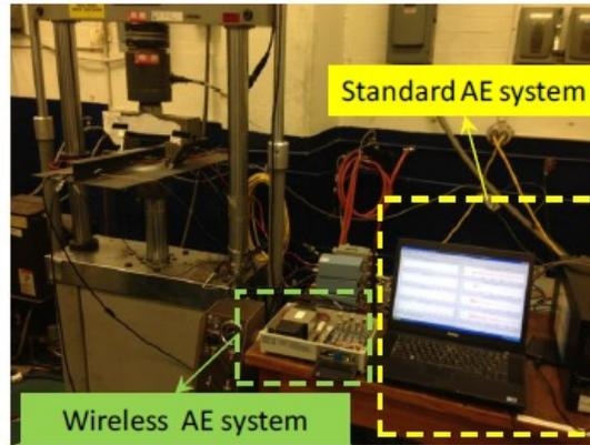
Figure 3. Three point bending AE test comparing the 1284 and a standard AE system.
