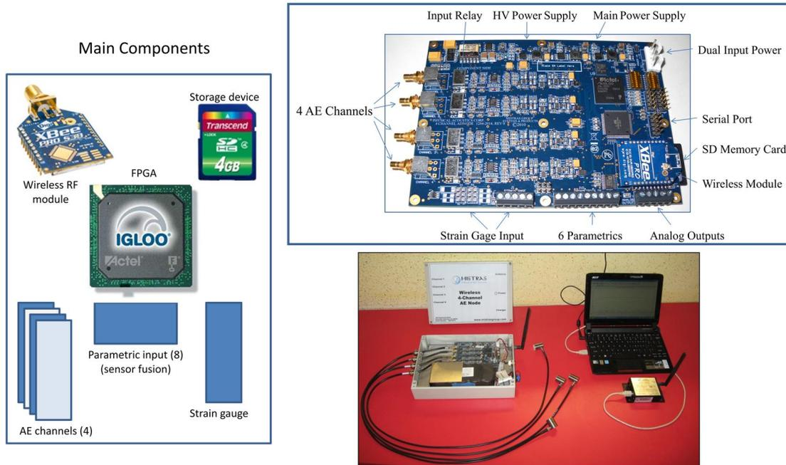
Figure 1. Components of the 1284 (4-channel wireless node), picture of the board (Rev 1.0) designed at Mistras, and the whole system connected to a laptop computer via a base station.
