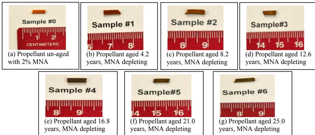
Figure 5. Photos of propellant samples that have not been aged (sample #0) and samples accelerated aged up to 25 years
