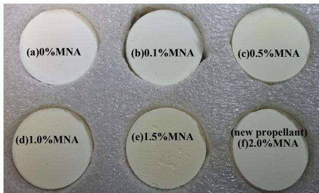
Figure 8. Photo of laboratory samples that have (a) 100% Aluminum Oxide ( $\text{Al}_2\text{O}_3$ ), (b)  $\text{Al}_2\text{O}_3$  & 0.1 % MNA, (c)  $\text{Al}_2\text{O}_3$  & 0.5 % MNA, (d)  $\text{Al}_2\text{O}_3$  & 1% MNA, (e)  $\text{Al}_2\text{O}_3$  & 1.5 % MNA, and (f)  $\text{Al}_2\text{O}_3$  & 2% MNA
