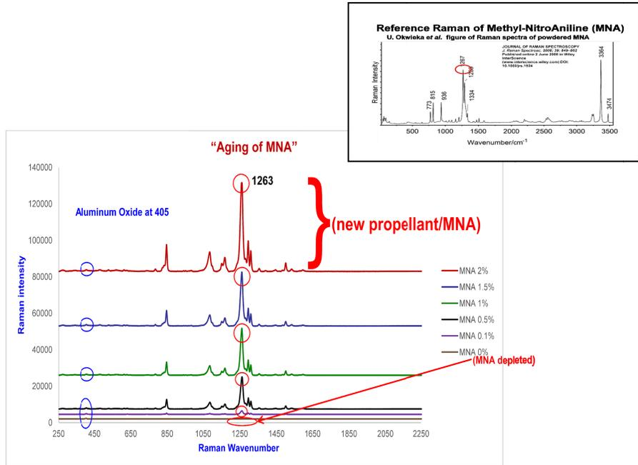
Figure 9. Measured results indicative of Raman spectrums for the simulated propellant samples
