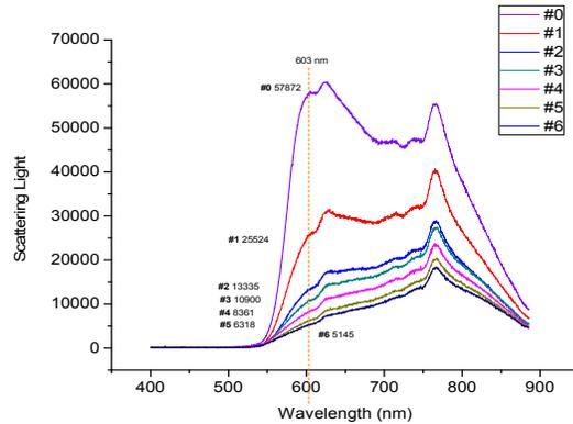
Figure 6. Measured results showing absorption spectrums for samples of un-aged propellant (sample #0) and propellant samples that experienced up to 25 years of accelerated aging
