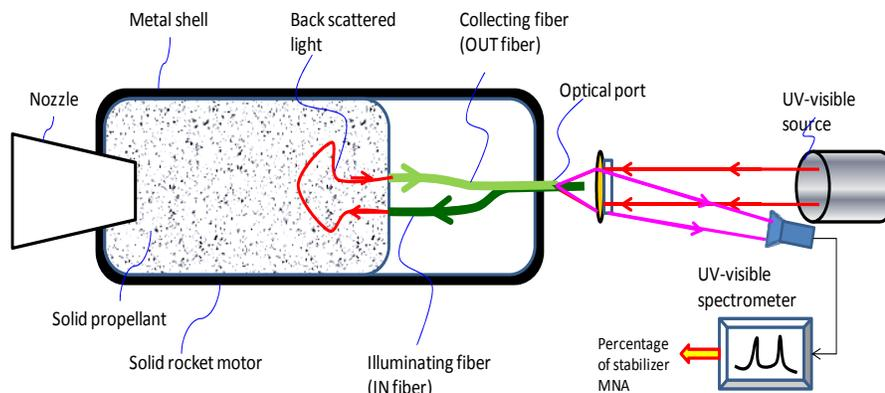
Figure 3. AMRDEC patented fiber optic spectroscopy method for measuring light intensity during heavy absorption of light by MNA, particularly at the UV/blue spectral
