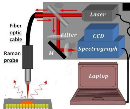
Figure 7. Fiber optic spectroscopy method for obtaining Raman spectrum results for propellant stabilizer (i.e., MNA)
