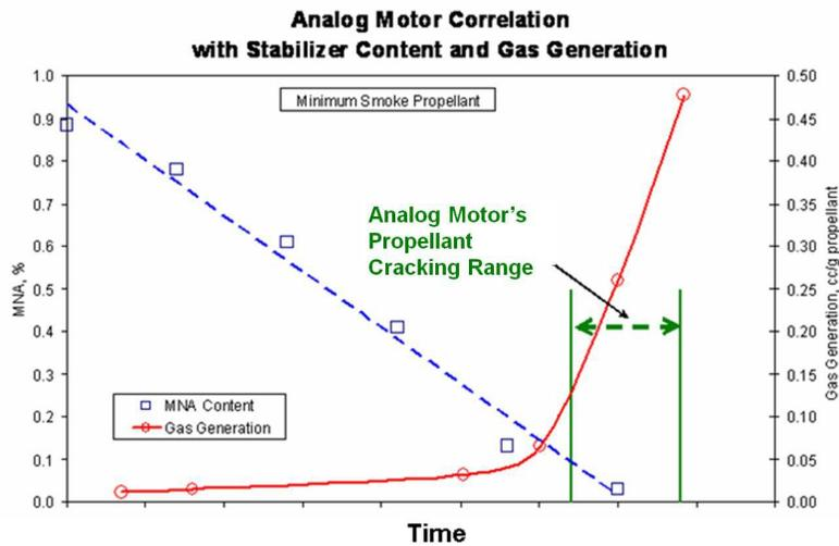
Figure 1. Stabilizer depletion (dash line) versus propellant generated off-gassing
