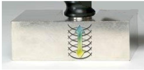
Figure 11. Acoustic sensing technique equating thickness to time it takes for the wave to pass through material (Reference Olympus Manual, DMTA-10022-01EN-Rev.B, October 2013)
