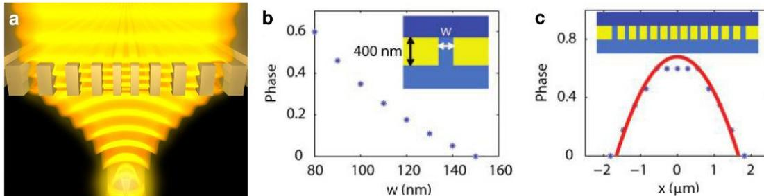
Figure 4. (a) Planar cylindrical lens formed by an array of slits in a metallic substrate. (b) The slit width determines the phase delay experienced by the channel-waveguided light. (c) A parabolic phase front is established, achieving focusing in the near-field at a distance of 5.3 mm behind the lens for a wavelength of 637 nm. Figures (b) and (c) adapted from Ref. 58, © 2009 ACS.
