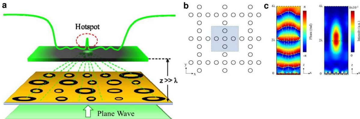
Figure 5. (a) Metamaterial aperture arrays designed to create super-oscillatory hotspots in a plane behind the structure. (b)-(d) Arranging the ring apertures in a sparsely arranged array breaks the symmetry and allows different local phase delays resulting in a curvature of the transmitted light. Figures adapted from Ref. 64, © 2013 OSA.
