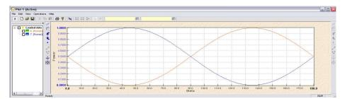
Fig. 4. Output power at the left side (red) and the right side (blue). Since the polarizer placed on the right side is oriented  $45^{\circ}$  clockwise with respect to the one on the left, there is a maximum transmitted power at an imposed field rotation of  $45^{\circ}$  (clockwise) passing from left to right and a minimum entering from the
