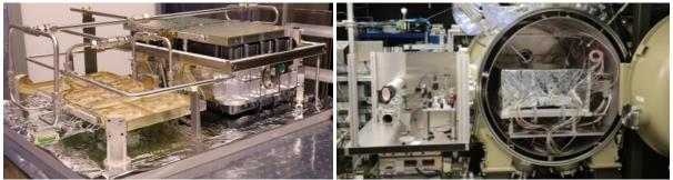
Fig. 7: Left: Laser in preparation for Thermal Vacuum testing; Right: test facility with integrated laser and external test setup for online laser performance measurement
