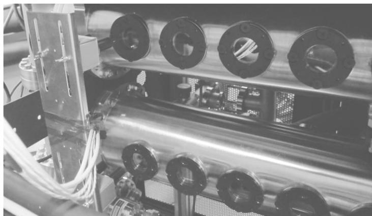
**Fig. 4.** Picture of the two vacuum tubes with its measurement windows and the mounting bracket with the two detector pairs on the left side
