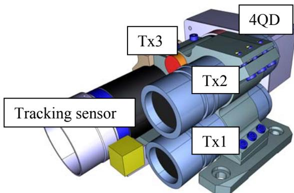
Figure 2: Optical bench of the OSIRIS payload
