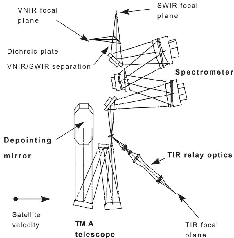
Figure 4 : PRISM Optical Architecture - The Earth is towards the reader.
