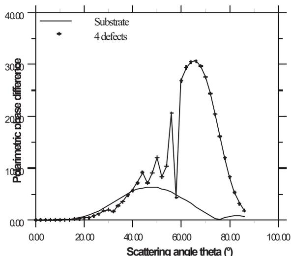
**Figure 10:** Simulation of a 2 nm rough interface with 4 defects (diameter 4 $\mu$ m, 10 nm high)
