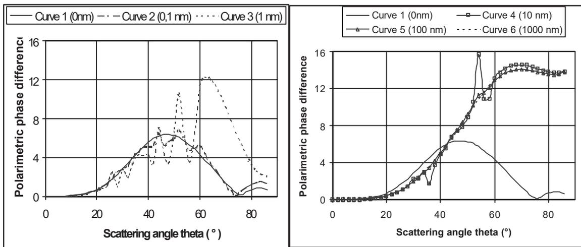
**Figure 8:** Calculation of polarimetric phase difference in the case of a 8H high index layer ( $\text{Ta}_2\text{O}_5$  Ion Plating) deposited on a 2 nm rough glass substrate. The layer brought roughness is 0 nm (curve 1), 0.1 nm (curve 2) and 1 nm (curve 3).
