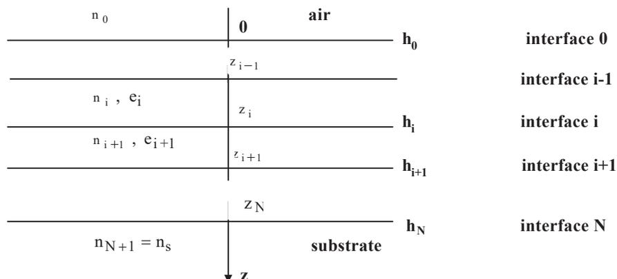
**Figure 7:** Definition of the opto-geometrical parameters of a multilayer.  $n_i$  and  $e_i$  are respectively for the index and the thickness of the layer number  $i$ .
