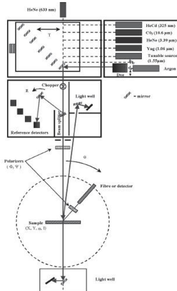
**Figure 1:** Experimental set-up at Institut Fresnel – Marseilles
