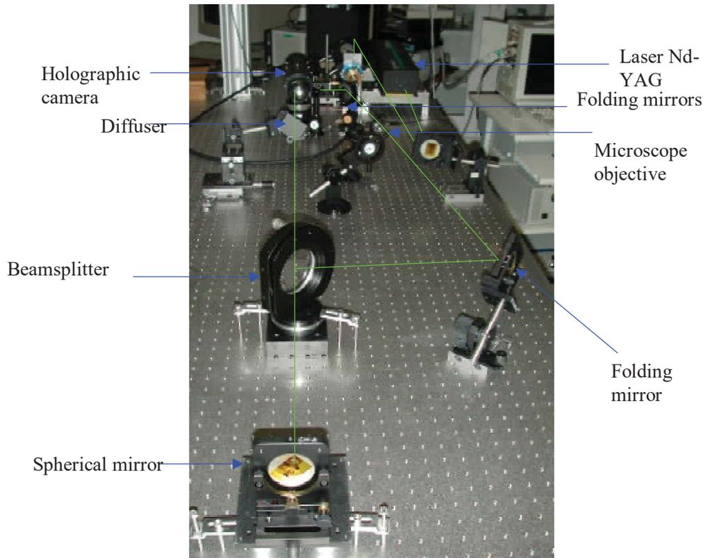
Fig 2 : Picture of the Breadboard experiment
