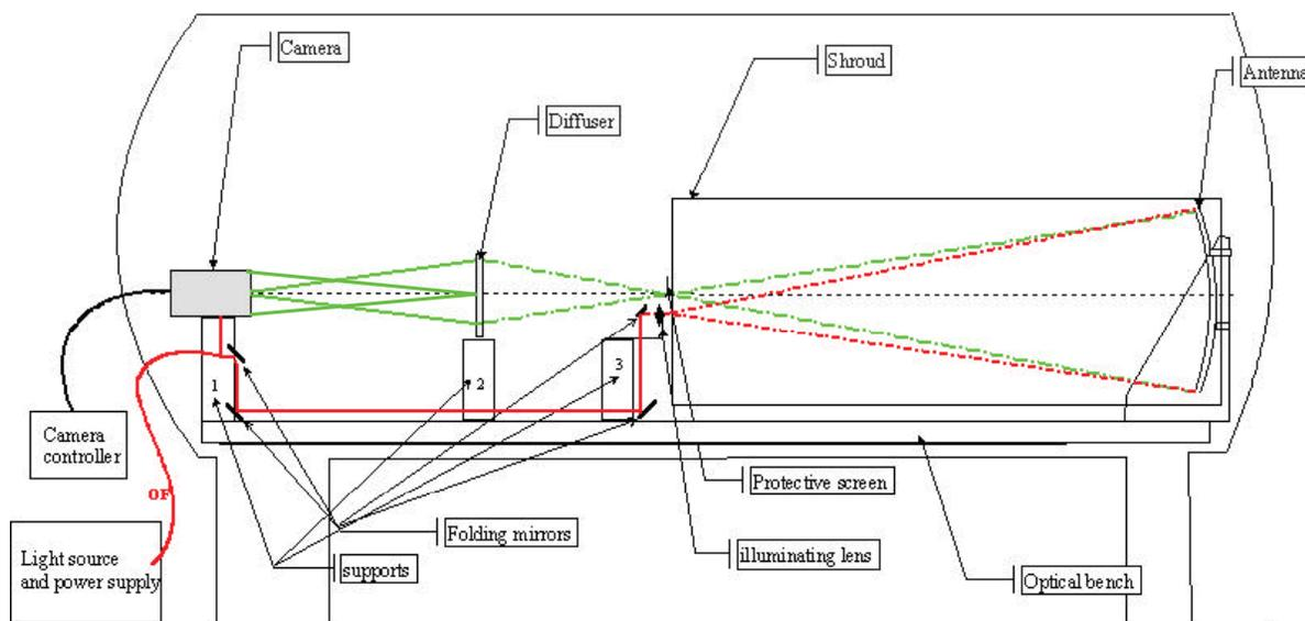
Fig 8 : Certification test layout
