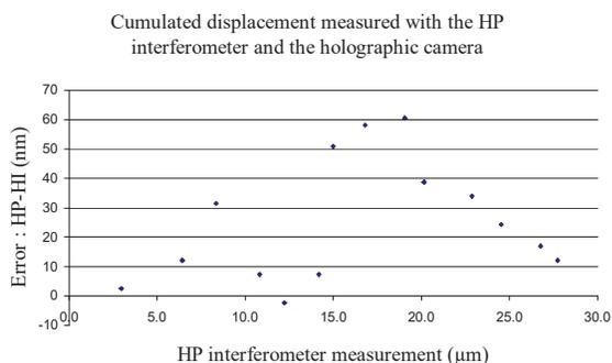
Fig 5 : Holographic camera calibration with a commercial interferometer of displacement of several tenth of µm.
