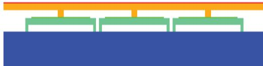
Fig. 2: Structure of micro-deformable mirror
