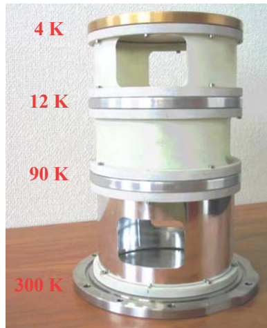
Fig. 2 Photograph of band 9 cartridge structure. Design is made by Rutherford Appleton Laboratory (UK).
