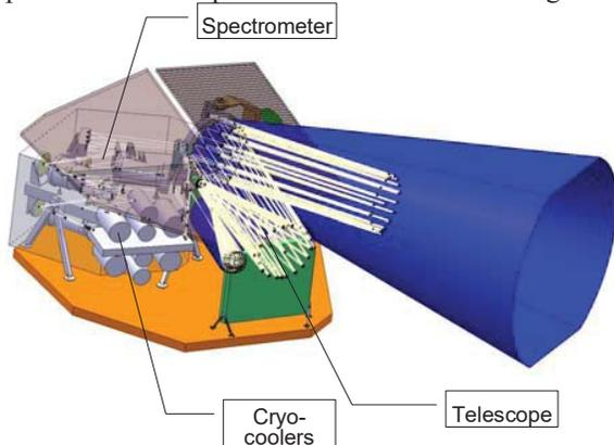
Fig. 4. Optical unit MTG IRS (dispersive option)
