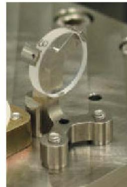
Fig 4: Glued fold mirror
