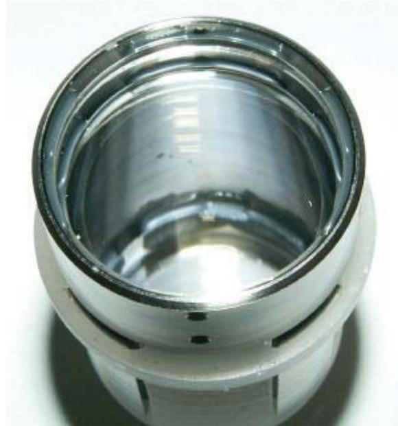
Fig. 6: Successful gluing of three lenses
