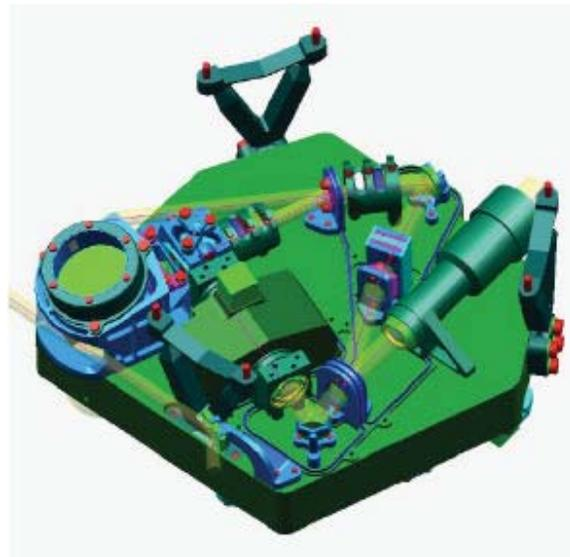
Fig. 1: Opto-mechanical layout of the TRO (stray light covers removed)
