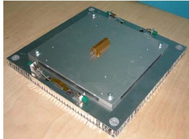
Fig. 5. Smart Panel Test coupon for verification of MAIT, functional and environmental testing
