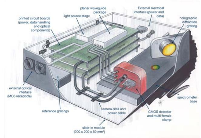
Fig. 11. 3D sketch of the Interrogator Unit
