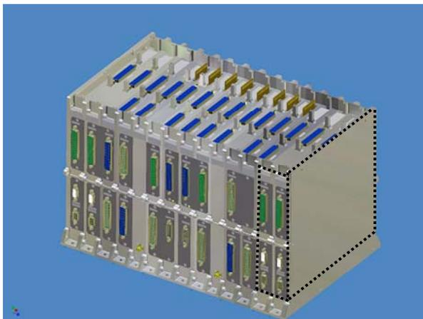
Fig. 10. Potential position of Interrogator Unit in a standard On-Board Computer (OBC) from Astrium
