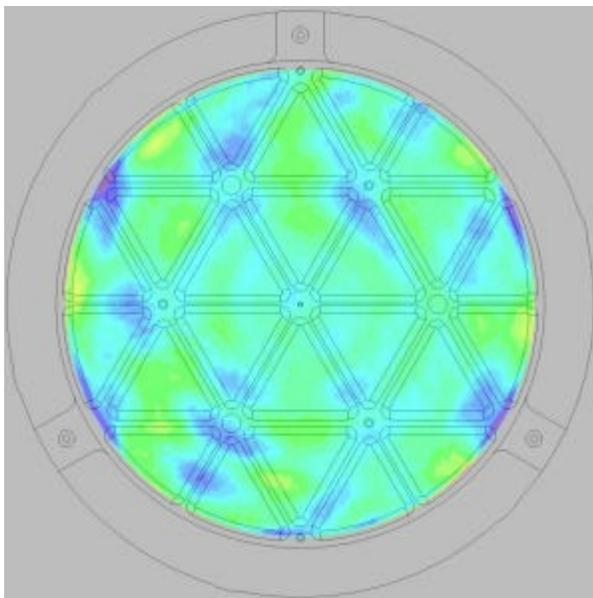
Fig. 6. Residual irregularities of the 300 mm M7 layered on a mechanical drawing of the back of the mirror. The relation between light weight pockets and print through is visible but insignificant: Residual irregularities are in the range of 4nm RMS, while surface roughness is still around 1 nm (Ra). The OPD map (created with Intellwave) shows the remaining irregularities, with tilt, focus, astigmatism, symmetric and asymmetric subtracted.
