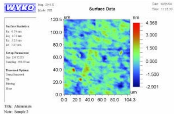
Fig. 2. Polished sample, Ra= 0.59 nm
