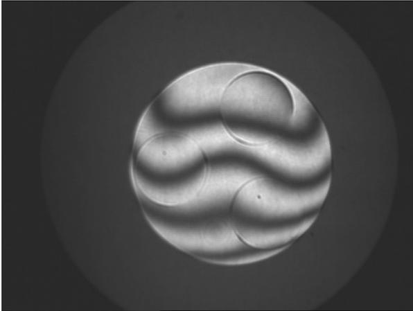
Fig. 3. Fringe pattern of the concave 200mm mirror after polishing (three segments visible).
