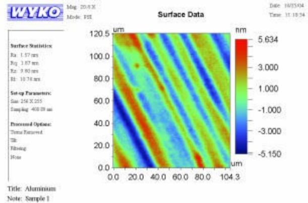
Fig. 1. Diamond turned sample, Ra= 1.57 nm.
