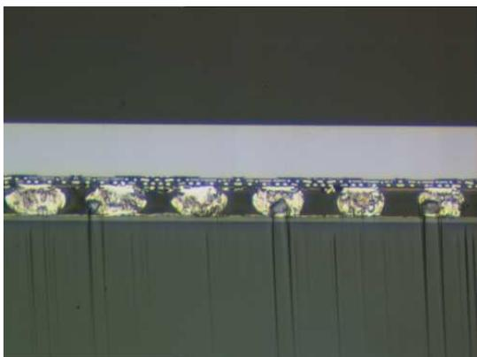
Fig. 12: SEM image of a polished readout circuit hybridized to an AlGaIn on sapphire 2D array.
