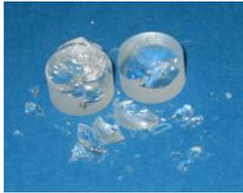
Fig. 3: Breakage after shearing stress
