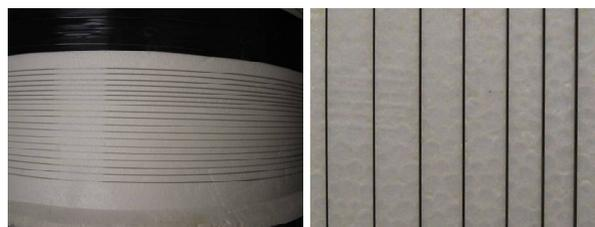
Fig. 1. Mono-index TeGeGal fiber on drum
