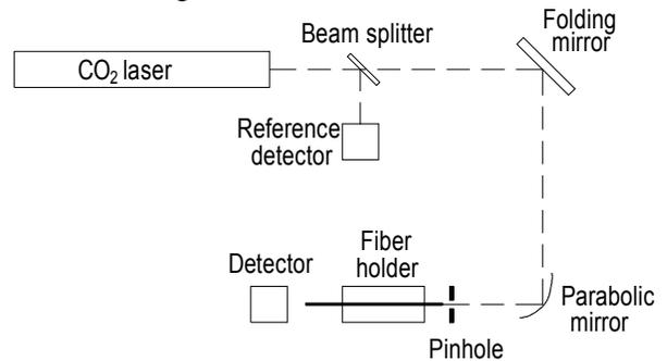
Fig. 3. Pulsed CO<sub>2</sub> laser set-up for fiber attenuation measurements at 10.6 μm
