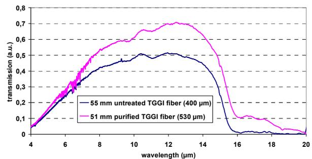
Fig. 4. Comparison of spectral transmission of a 5 cm fiber of purified and non-purified (untreated) TeGeGal mono-index fiber
