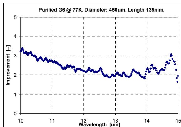
Fig. 6. Factor of improvement in transmission of a TeGeGal fiber at liquid nitrogen compared to room temperature
