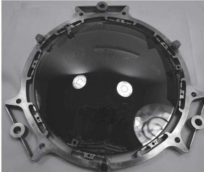
Figure 5-1 Assembled AR with the CaF<sub>2</sub> spherical dummy lens
