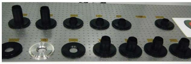
Figure 5. Picture of all the manufactured occulter.
