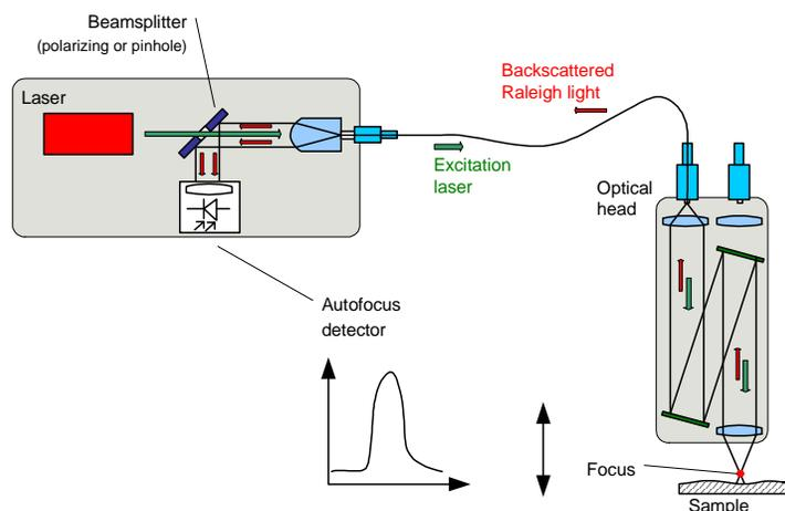
Fig. 7. Autofocus working principle
