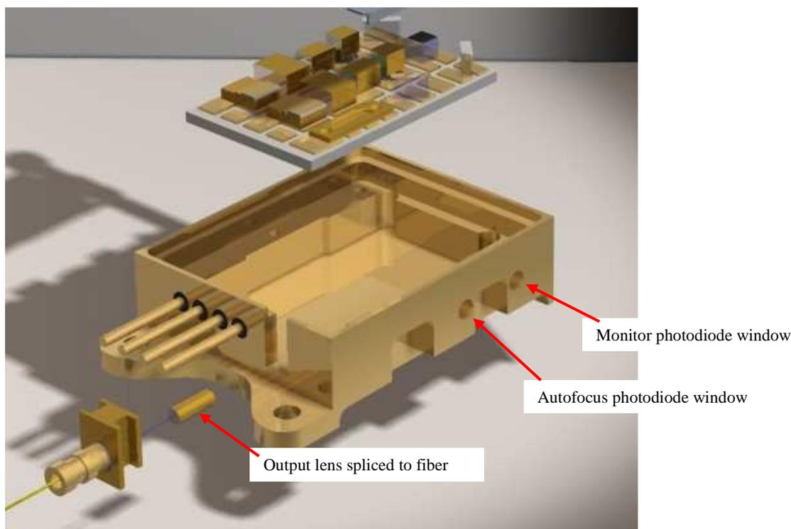
Fig.1, Outline of the laser housing with its optical interfaces
