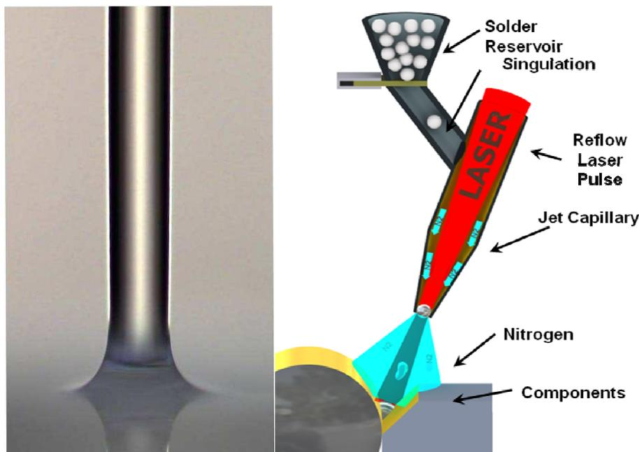
**Fig. 2**, Example of the splicing technique (left) and diagramme of the solderjet bumping mechanism (right) from the Fraunhofer Institute.
