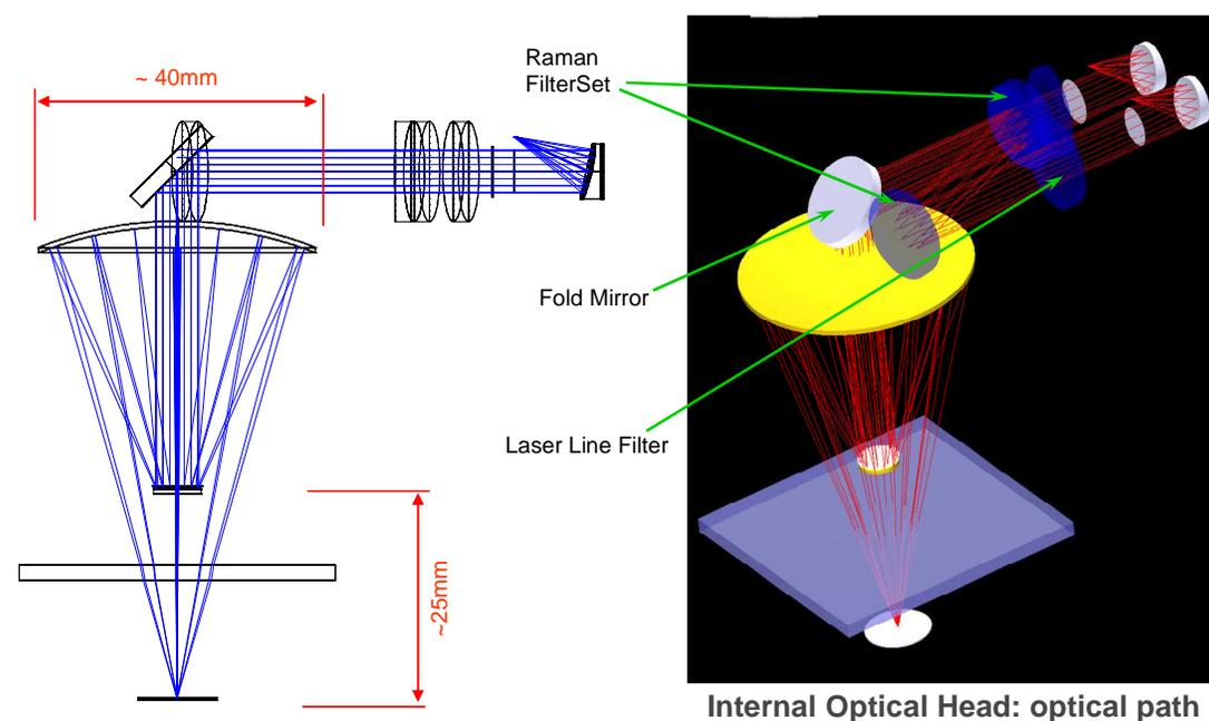
Fig. 5, Optical layout for achieving the high back focal distance
