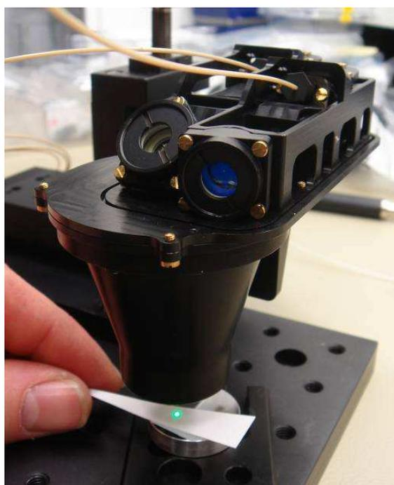
Fig. 6, Raman optical head breadboard during alignment (cover removed)
