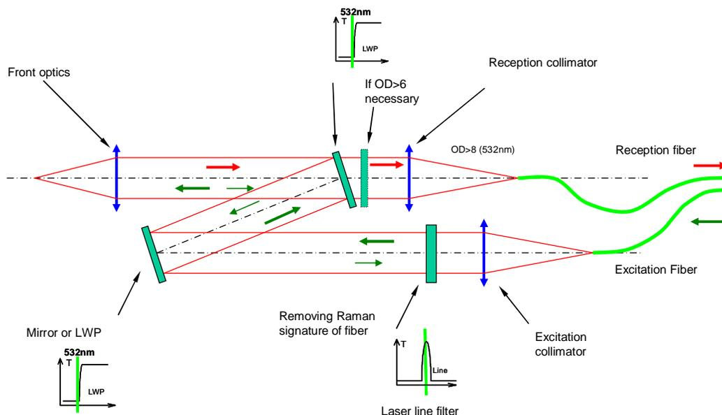
Fig. 4, Filter concept of the optical head for removing fiber and Laser signatures in the excitation path and for blocking the backscattered excitation wavelength in the reception path
