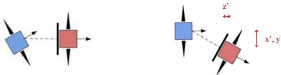
**Fig. 5.** Two possible cases (left: C-S/C (blue) off-pointed; right: O-S/C (red) translated) leading to similar OPS measurements.
