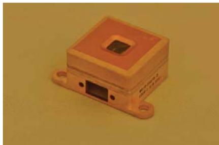
Figure-3. FSS quadrant detector module for BepiColombo
