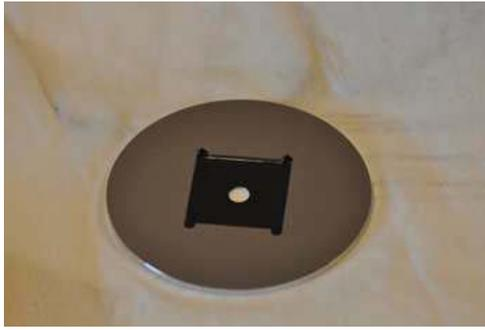
Figure-8. Special tooling to enable spin-coating of the square sapphire substrates.
