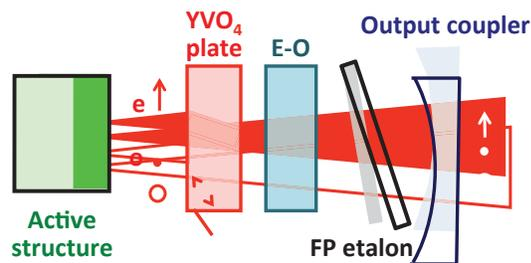
Experimental setup of the dual-frequency VECSEL
