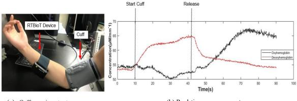
(a) Cuff experiment setup Figure 4. Real-time measurement of hemoglobin changes by using cuff machine
