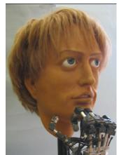
**Figure 4:** A humanlike robot made with Frubber skin making it lifelike. The head (created by David Hanson) and the hand (created by Graham Whitely) shown in this photo are located in the author's NDEAA lab at JPL.
