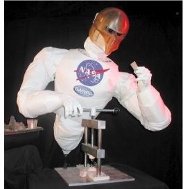
**Figure 8:** The Robonaut I is remotely controlled to perform physical tasks by mirroring the actions of a human (image: NASA Johnson Space Center).
