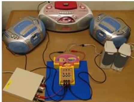
Figure 9. A simplified demonstration set for wavelength multiplied optical communication with a white-color LED.
