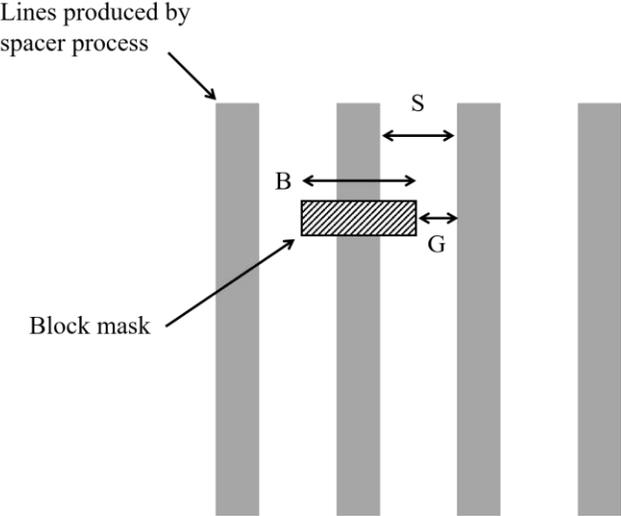
Figure 1. Schematic of block masking for a line-space pattern generated using a spacer process.
